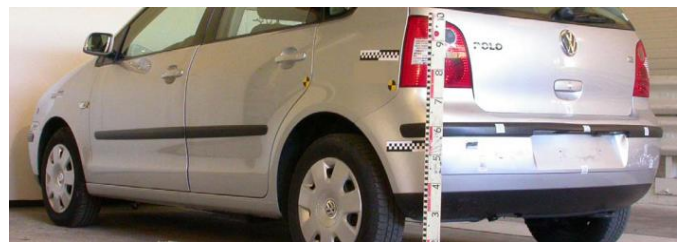
'AGU-Datenbank, Versuch Nr. SG_02' _delta \Delta v_{\text{Kompression}} = 5,0 km/h
